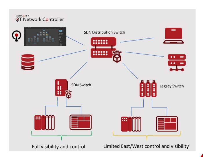
The Veracity OT Network Controller simplifies network management, provides robust deny by default security, and supports a zero-trust network architecture.
